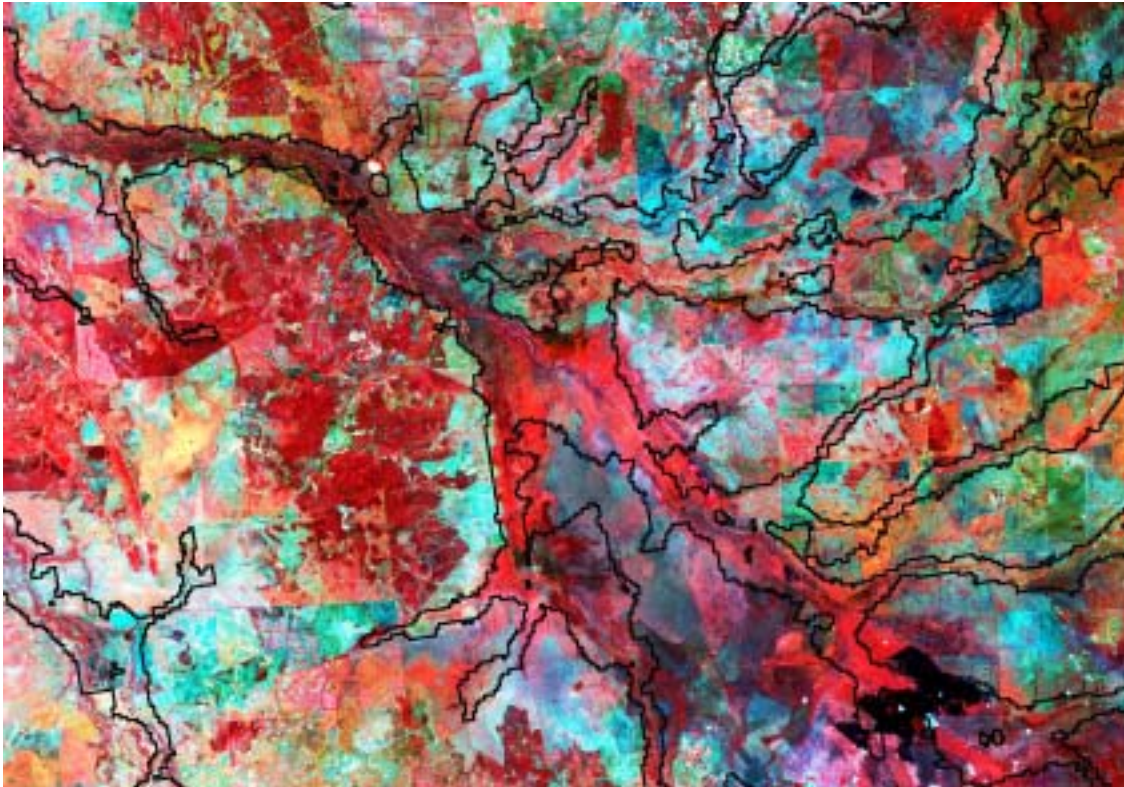
Figure 14: A Landsat TM image of part of the Sutor River catchment, Queensland. The black lines delineate modelled 25-year flood extents. The image has been transformed using the LS-FIT algorithm in the ENVI image processing package to find pixels containing features characteristic of clay minerals (Research Systems, 2000). The red band shows the LS-FIT clay residual value (with brighter values suggesting higher clay content), green shows TM band 2, and blue shows TM band 1.
